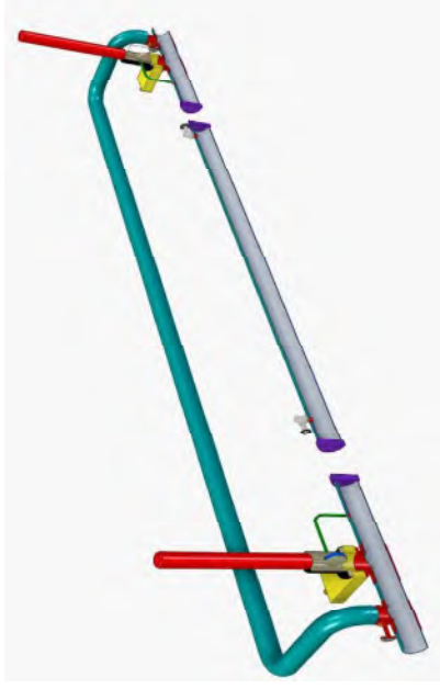
Fig. Upstream Stopple Plug Retraction
