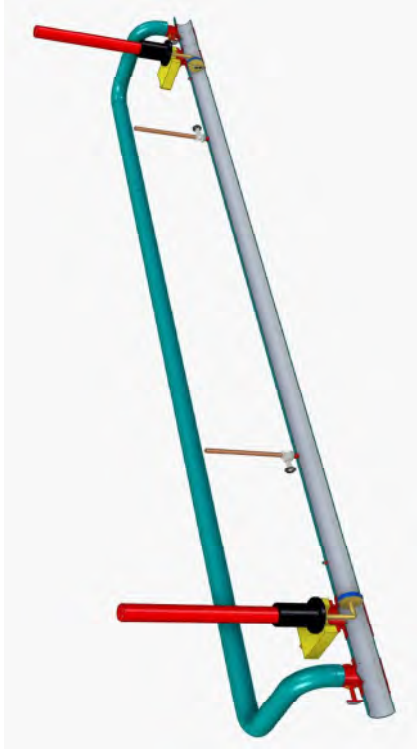
Fig. Venting of Isolated section using 4" Weld-olet Fitting.
