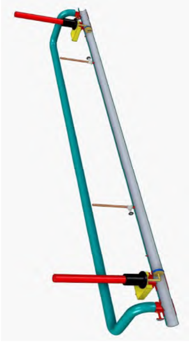
Fig. Venting of Isolated section using 4" Weld-out Fitting.
