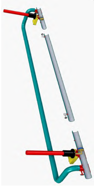
Fig. Venting of Isolated section using 4" Weld-olet Fitting.
