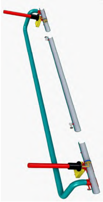
Fig. Venting of Isolated section using 4" Weld-out Fitting.
